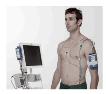
Fig 6. Low cost compact wireless ECG sensor. © Isansys Lifecare
