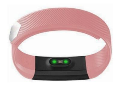
Fig 4. The blood flow record by Ir technology for heart rate check are low accuracy not support heart pulse.
